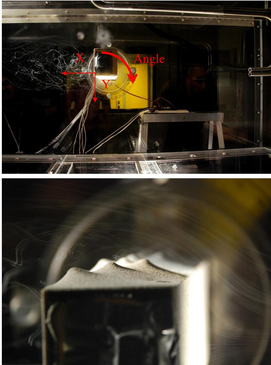
**Figure 6. The test section of the wind tunnel with the helium bubble visualization device on. A wide-angle image showing the flow from right to left (top). The building is placed in the middle of the test section. Downstream it is possible to see the trajectories of the helium bubbles mapping the flow and the vortices generated by the building interference. A close-up of the model with the patterns completely out (bottom).**
