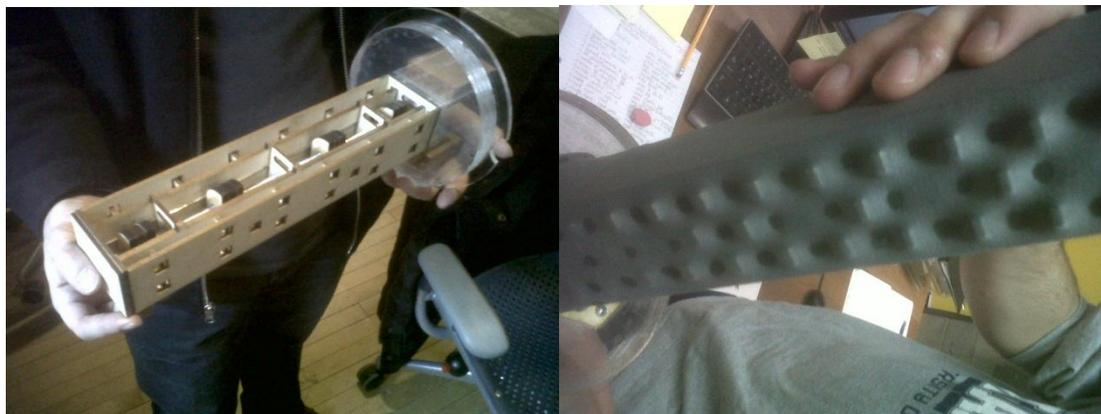
**Figure 4. Model 3 basswood armature (left) and covered with Spandex (right)**
